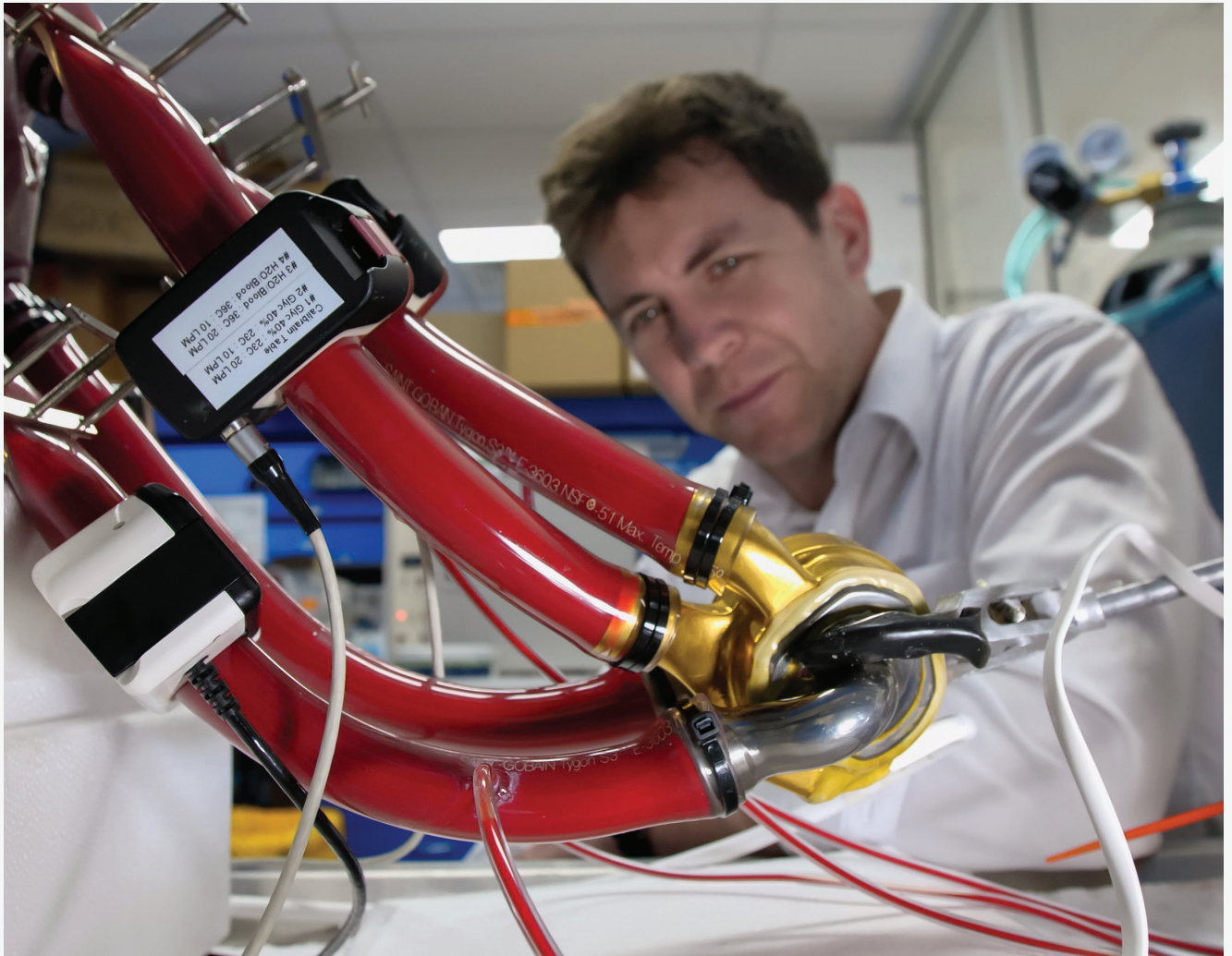
BiVACOR Total Artificial Heart Blood Loop Test with Daniel Timms, PhD, Founder & CTO. Credit: BiVACOR
